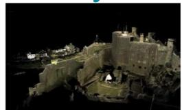
Sophisticated 3D laser scanning technology has been used by a UK TV Channel 4 to create high-definition fly-though animations to map development of advanced fortifications around Mont Orgueil Castle in Jersey. A survey team from Digital Surveys captured hundreds of millions of millimetre-accurate measurements for Channel 4's flagship programme Time Team, which has been uncovering the archaeological mysteries of the British Isles since 1994.
