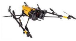
Topcon Positioning Group has added a rotary-wing UAS to its mass data-collection solutions line for the European marketplace. The Falcon 8 – powered by Ascending Technologies – is designed for inspection and monitoring as well as survey and mapping applications.
