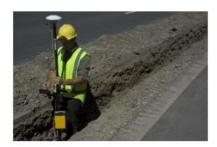
Trimble (CA, USA) has introduced the GPS Pathfinder ProXRT receiver, a flexible GNSS receiver for GIS data collection and mapping. The receiver combines a high- performance GPS receiver with Trimble H-Star technology, OmniSTAR correction capability, and optional GLONASS capability to provide various levels of positioning accuracies, from submetre to decimetre (10cm) accuracy.
