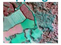
DroneMetrex has announced that near-infra-red (NIR) mapping data has been captured with the TopoDrone-100. The radiometric quality has been achieved because DroneMetrex specialists performed the necessary camera modifications and have designed the external filters specifically to match the requirements for accurate, discriminative vegetation mapping. According to DroneMetrex, this is the first time in the UAV's mapping history that NIR imagery has been captured at this level of quality.
