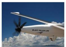
Silent Falcon UAS Technologies has unveiled a fully integrated photogrammetric sensor package that flies aboard the solar-electric-powered Silent Falcon UAS. Incorporating the custom Falcon XCAM-A camera system, Pix4D processing software and LizardTech compression technology, the Silent Falcon photogrammetric package is designed to capture mapping-quality image data on long-endurance, extended-range UAS missions.
