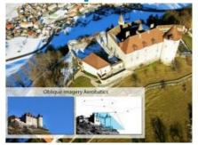
senseFly's drones eBee and swinglet CAM, both designed for mapping missions, are capable of capturing oblique images quickly to complement a mapping project or to add additional documentation. This patent-pending technology is based on a propriatary control algorithm that takes oblique images of photo targets without the need for a camera gimbal, enabling senseFly's ultralight mapping drones to take aerial shots with up to 45° inclination from the photo target.
