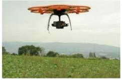
Leica Geosystems, Aibotix and Headwall Photonics have introduced an integrated high performance airborne sensor solution utilising a hyperspectral imager and the Aibot X6 UAV. The Nano-Hyperspec sensor was optimised in terms of size, weight, and power to enable the aerial acquisition of all spectral and spatial data within the scene of interest. A UAV with integrated Headwall sensor has already been successfully flown and will be presented at this year's Intergeo in Berlin.
