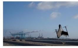
Van Oord is using Marlyn Cobalt survey drones to ensure design conformance and increase safety at the Port of Rotterdam, the largest container port in Europe. The Dutch port is currently expanding its quays and retaining walls to increase its container transshipment capacity.
