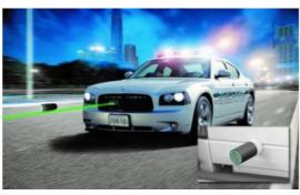
US police officers are trialling a new piece of GPS technology called StarChase to reduce risks associated with pursuits. The StarChase system uses a compressed air launcher mounted in the grille of a police vehicle to launch a GPS device, which adheres to a suspect's vehicle. The system can then track a suspect's vehicle in near real time on a secure map. Once tagged, officers can fall back and coordinate a tactical "safe stop" to apprehend the suspect.
