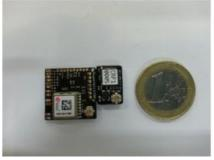
Researcher Bart Remes and his team of the Micro Aerial Vehicle (MAV) Laboratory at the TU Delft (The Netherlands) faculty of Aerospace Engineering have designed, built and tested the world's smallest open source autopilot for small unmanned aircraft. A smaller and lighter autopilot allows these small flying robots to fly longer, fit into narrower spaces or carry more payloads, such as cameras.
