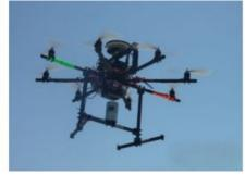
Phoenix Aerial Systems, a manufacturer of unmanned aerial platforms, has developed and demonstrated what it says is the world's smallest and lightest UAV Lidar platform. Weighing less than 10kg, the new Lidar platform called the Phoenix AL-2 combines the latest UAV, Lidar and GNSS technology into an accurate and safe micro-mapping solution.
