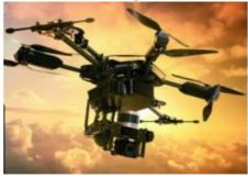
XactSense has developed a new platform for low-altitude aerial mapping using the newly released Velodyne Lidar VLP-16 puck. According to the American company, which is based in Rhode Island, drone mapping for the masses is now here. The new multi-laser puck builds on Velodyne's reputation for small, lightweight Lidar, and XactSense's founder, Andy Trench, described this next-generation sensor as a game changer since companies of all sizes can now afford to utilise the emergent drone technology.
