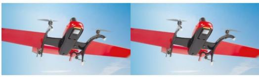
In a new partnership with YellowScan, FIXAR's flagship UAV model, the FIXAR 007, will be upgraded with a YellowScan Lidar system. YellowScan is one of the leading designers of next-generation Lidar solutions, while FIXAR is a European developer of unmanned aerial vehicles.
