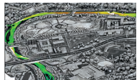
▲ Lidar-derived surface model of the Saint-Charles River, Pointe-aux-Lièvres Park, with bathymetry shaded by depth. (Image courtesy: Chris Miwa, NV5 Geospatial)
