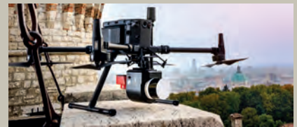
▲ The Scanfly v3 features a versatile, multi-platform design, tailored to accommodate a unified workflow across UAVs, land vehicles and even when worn as a backpack. (Image courtesy: 3D Target)
