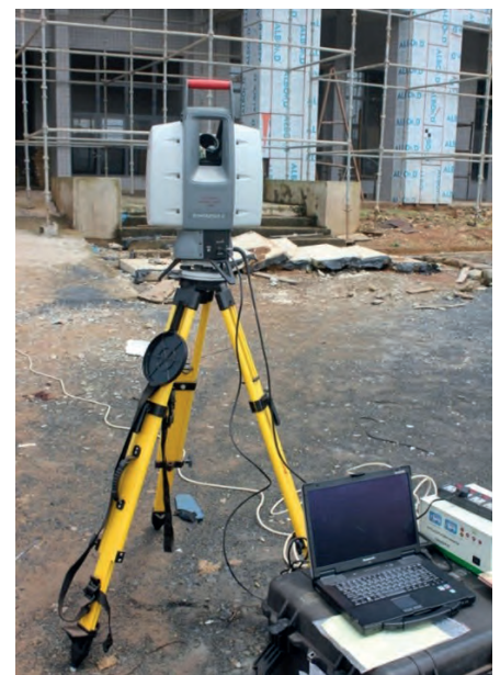
▲ Figure 1: HDS Leica ScanStation-2 TLS used for the 3D modelling of the offshore gas platform. (Author's own image)
