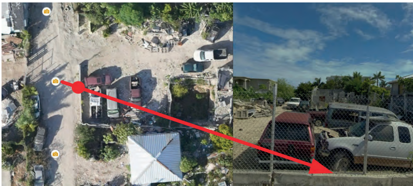
▲ Figure 5: Data capture in the Turks and Caicos Islands included PLACE Aerial (5cm aerial) and PLACE Ground (360-degree street view), engineering-grade data that can be used for measurements, coordinate identification, etc.
