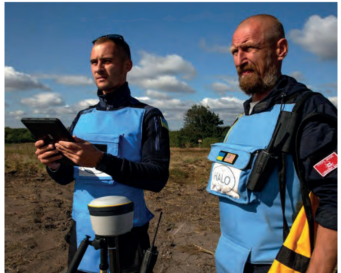
▲ A mine clearance team in Ukraine setting up a Trimble R2 GNSS receiver that is used to support landmine identification and clearance by mapping land at 2cm spatial accuracy.
