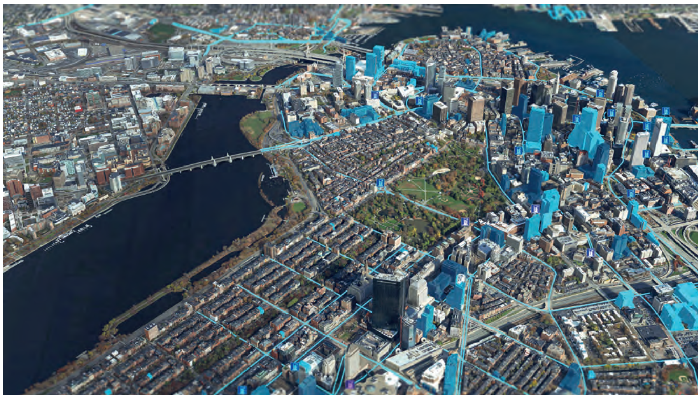
▲ Figure 5: Example of a reality mapping 3D model for the city of Boston, as the foundation for digital twins of cities. (Image courtesy: Bluesky and Esri)
