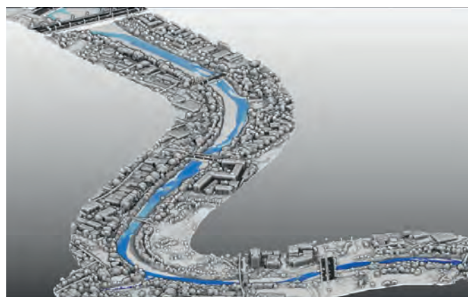
▲ Lidar-derived surface model of the Saint-Charles River, with bathymetry shaded by depth. (Image courtesy: Chris Miwa, NV5 Geospatial)
