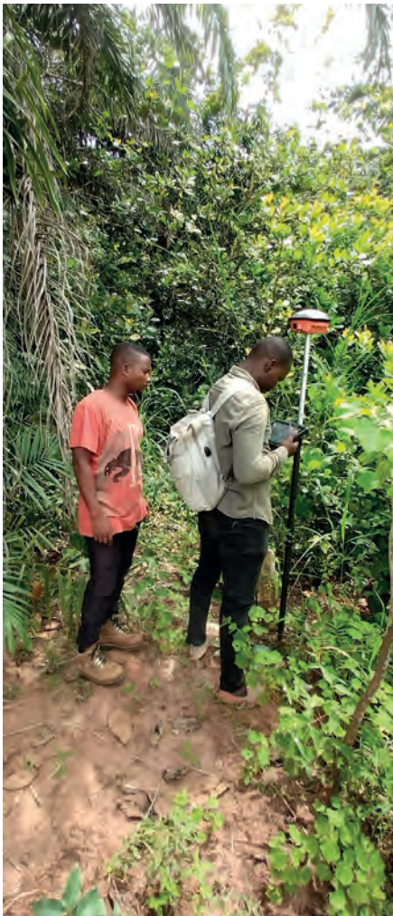
▲ Using a GNSS receiver to measure parcel boundaries.
