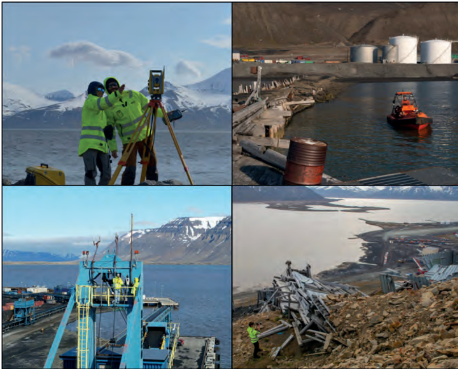
▲ Figure 3: The documentation process included land surveying with total station, image acquisition from a boat to document the old coal loading pier (Gammelkaia), laser scanning on top of the modern coal quay at Kapp Amsterdam, and image acquisition at mine entrances from the 1970s. (Courtesy: NIKU)
