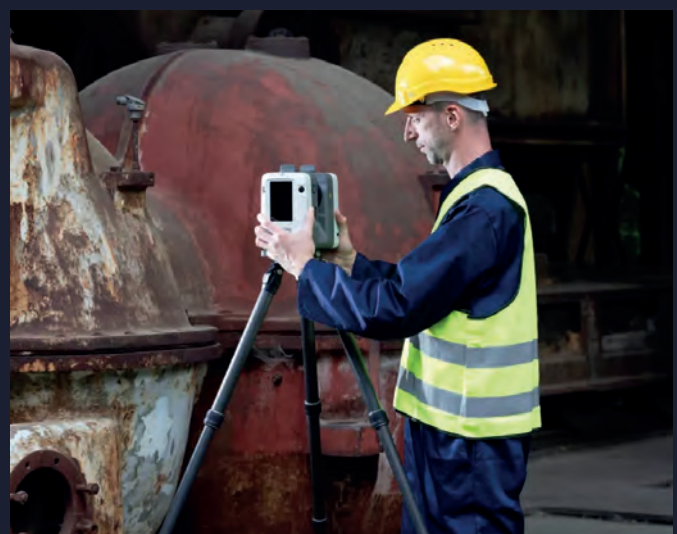
▲ The Artec Ray II 3D Lidar scanner is designed for digitizing large objects and spaces. (Image courtesy: Artec 3D)
