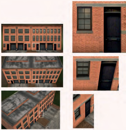
▲ Figure 3: Standard Maltese-cross oblique cameras are less capable of capturing facades of buildings that are not aligned with parallel flight lines.
