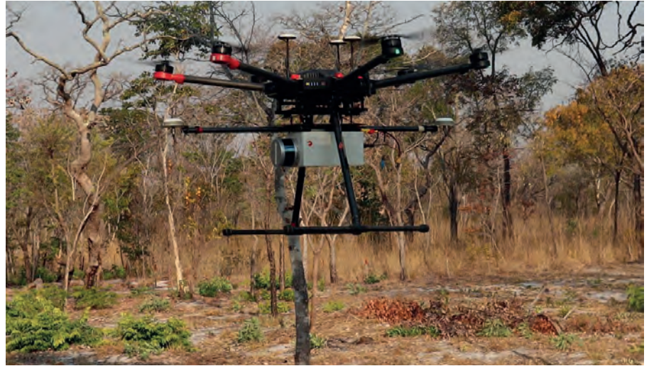
▲ Figure 4: The Routescene UAV Lidar system mounted underneath a DJI M600 Pro in Angola.
