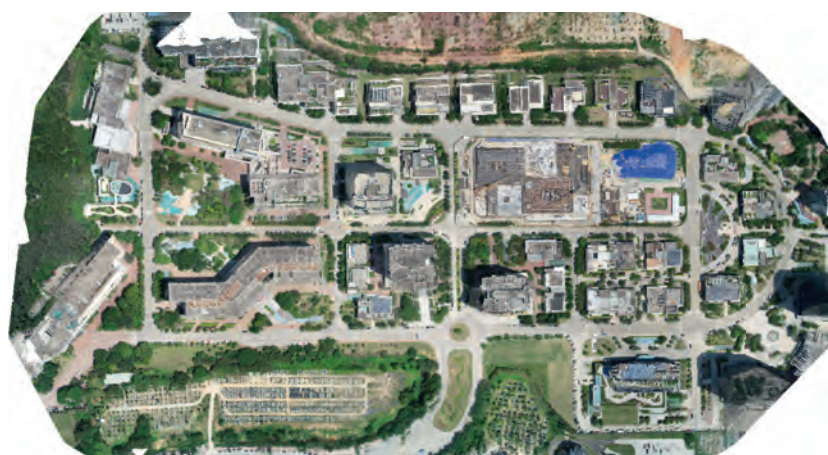
▲ Figure 3: DOM produced by Pix4Dmapper software.
