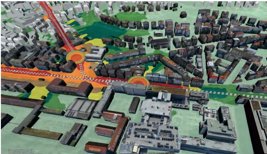
▲ Scenario 2: Noise from a tram is simulated as a moving volume bubble, with each layer portraying different decibel levels. (Image courtesy: Hexagon)
