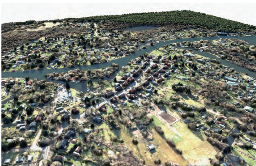
▲ Figure 1: Example of an AI-generated twin of the Earth's digital surface using Deeper's variation of the monocular depth estimation method.
