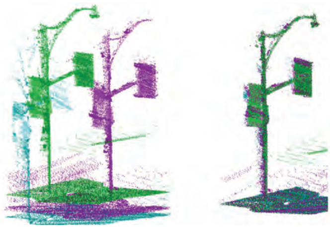
▲ Figure 5: Before adjustment (left) showing a lamp post double, and after adjustment (right) showing the aligned scans from two passes on the same road.
