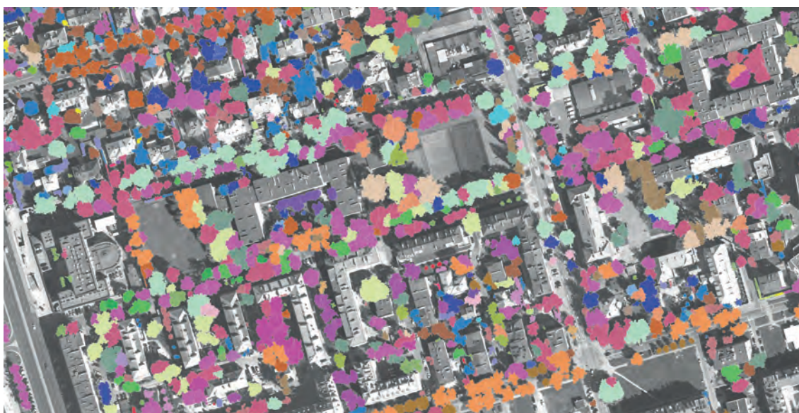
▲ Imagery derived from Warsaw's multisensor Tree Crown Map, showcasing the automated classification of tree species.
