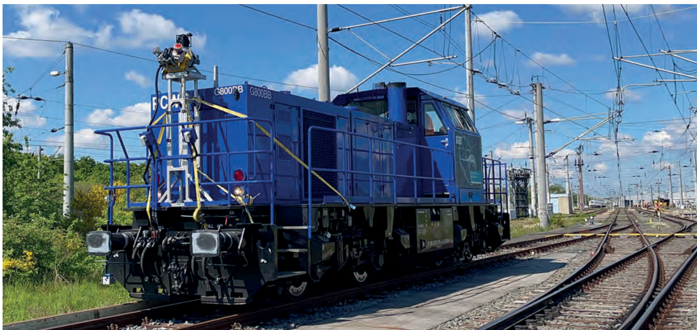
▲ The Trimble MX9 is the first vehicle-independent mobile mapping system officially approved by Deutsche Bahn for surveying tracks, points, clearances and topographic objects. (Image courtesy: Trimble)
