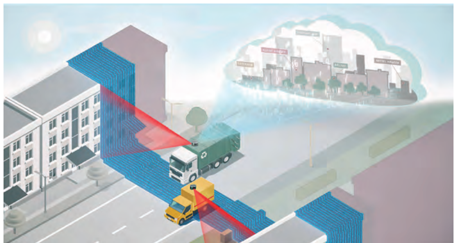
▲ Fraunhofer IPM is integrating a variety of sensors into a vehicle-mounted measurement box. The sensors collect data while the vehicle passes. The data is autonomously reduced and streamed in real time into the city's geodata service, where it is AI-processed and converted into geodata-compliant data formats. (Images courtesy: Fraunhofer IPM)
