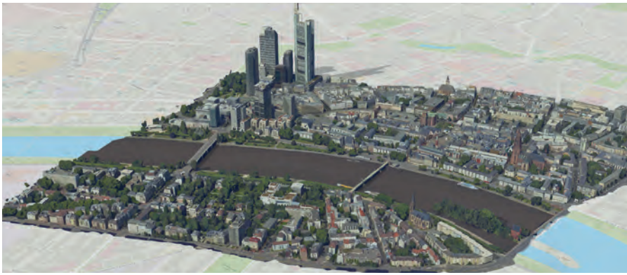
▲ Figure 3: Tiled 3D model (i3S/SLPK format) of Frankfurt city centre, served from the cloud and visualized in a web browser (output product from ArcGIS Reality Capture Studio tutorial; Esri, 2023).
