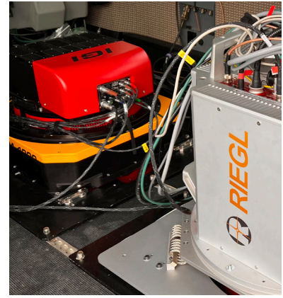
URBAN MAPPER-2 in dual-hatch C208 in Master-Slave Configuration
