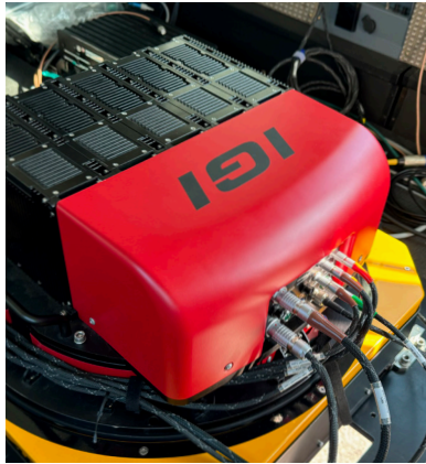
IGI URBANMAPPER-2 Performance installed in GSM-4000
