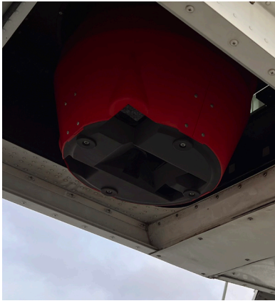
IGI URBANMAPPER-2 Performance installed in Cessna Caravan
