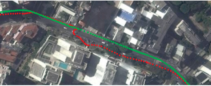
Multi-path mitigation in urban canyon: GNSS alone – red path ; imajbox® – green path
