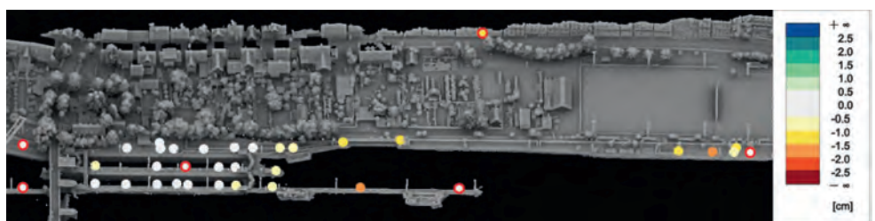
▲ Figure 5: Elevation differences of Lidar point cloud to signalized targets. GCPs are marked as red circles.
