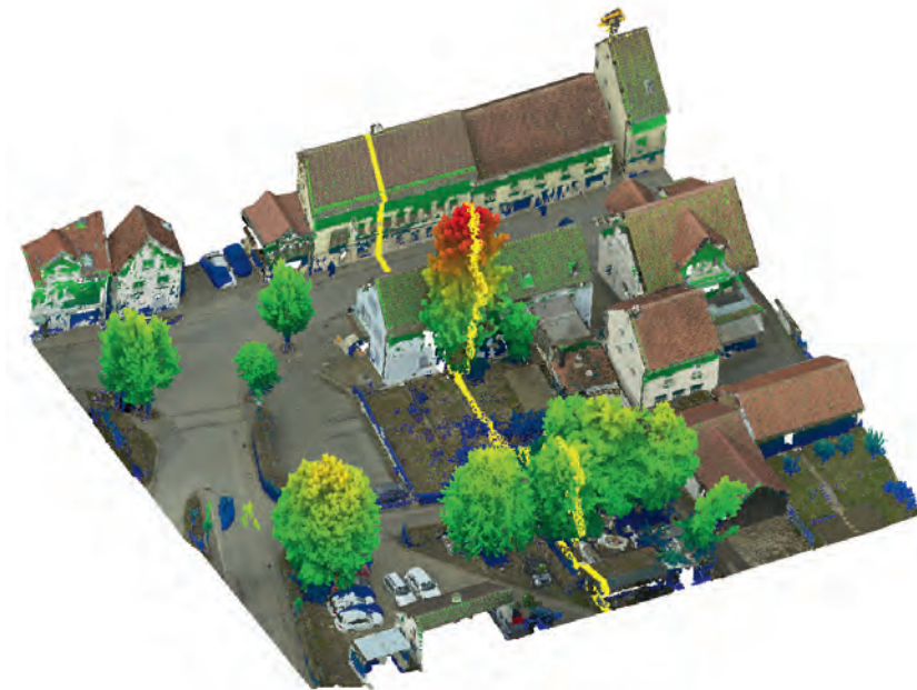
▲ Figure 8: Comparison of 3D points from MVS (RGB) and Lidar measurement (height coded). Yellow line defines profile depicted in Figure 9.
