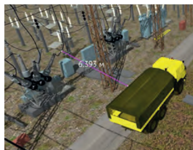
▲ Figure 6, Automatic tracking of the shortest distance between a moving vehicle and a high-voltage wire.
