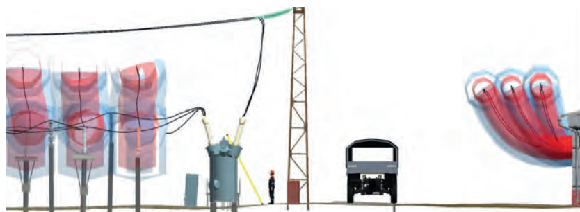
▲ Figure 7, Orthographic projection of a part of the 3D model for planning repairs.
