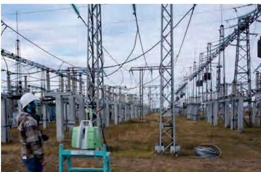
▲ Figure 1, Laser scanning of the power substation.
