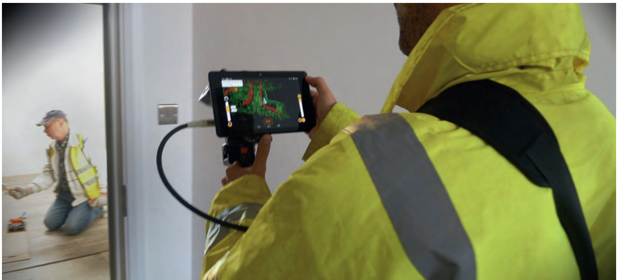
► Walking with the GeoSLAM ZEB-REVO on site.
