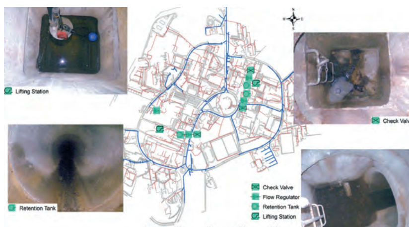
▲ Figure 4: Use of GIS to visualise the equipment of the storm-water system in the SunRise project.
