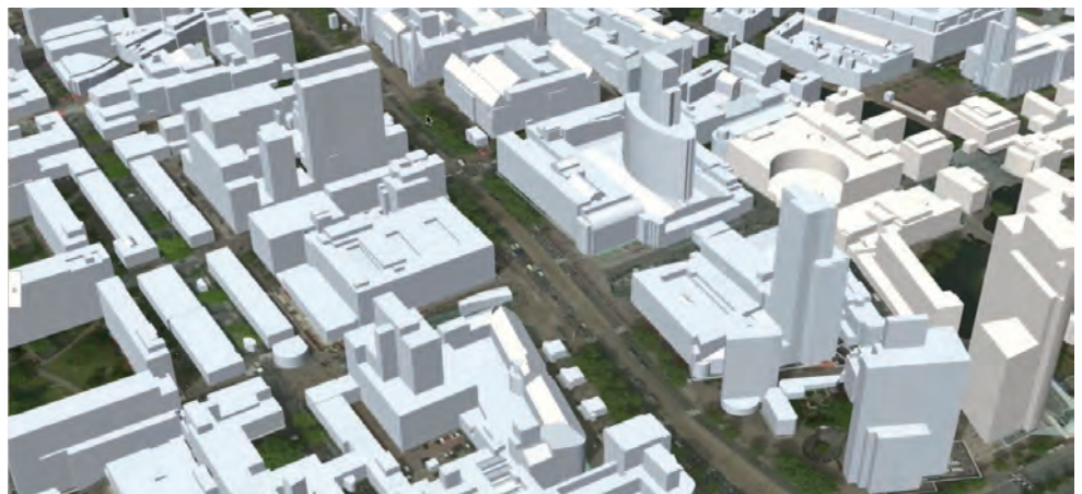
▲ Figure 4: 3D map at LoD1 of a part of Rotterdam automatically created by combining building footprints with airborne Lidar point clouds (source: Municipality of Rotterdam).
