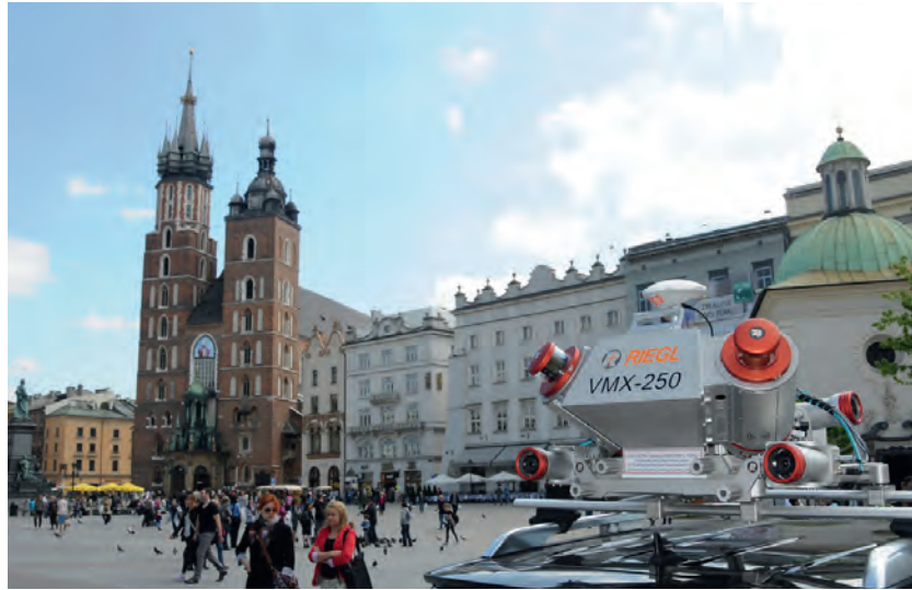
▲ Figure 3: A RIEGL VMX-250 mobile scanning system scanning the historic market square of Krakow, Poland (source: RIEGL, Austria).
