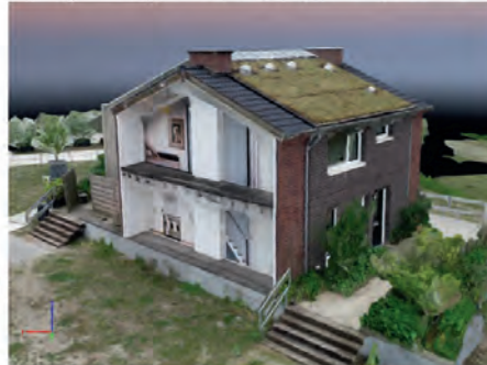
▲ Figure 10: Point clouds and meshes generated by SP software (left) and Pix4Dmapper.
